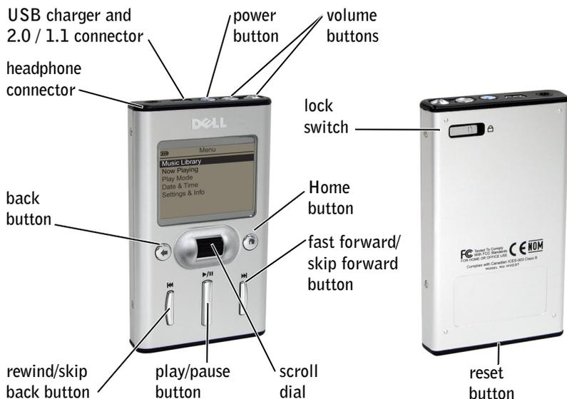
**POWER BUTTON** —Press and hold the power button for 2 seconds to turn the device on or off.
